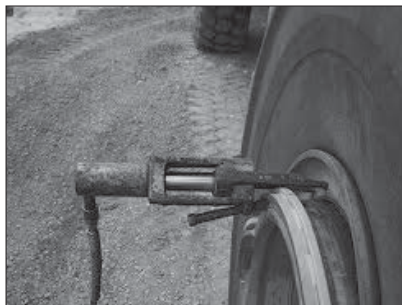
Hydraulic tire remover (rim flange push type) in operation.
